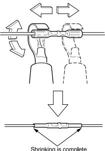
Shrinking is complete when sealant appears here.
