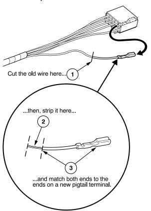
3. Select a pigtail terminal that matches the original wire at both ends (same kind of terminal and same diameter bare wire).
