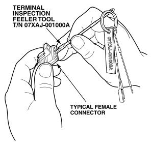
3. Compare the drag to the other terminals in the connector. If the drag is less, replace the terminal with a replacement terminal from the appropriate terminal repair kit.
