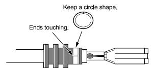
8. Inspect the quality of the wire crimp. If it has any of the following NO GOOD crimps, cut it off and start over.
