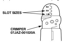
3. Strip the insulation off the end of the wire so the wire fits in the new terminal as shown. (If the wire has a wire seal, replace it with a new one from the kit.)
