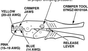
9. Insert one of the bare wires into the splice connector end that is in the crimper jaws. Push the wire all the way into the splice connector, and squeeze the crimper handles. Keep squeezing until the jaws touch, and hold it at that position until the ratchet clicks again.
