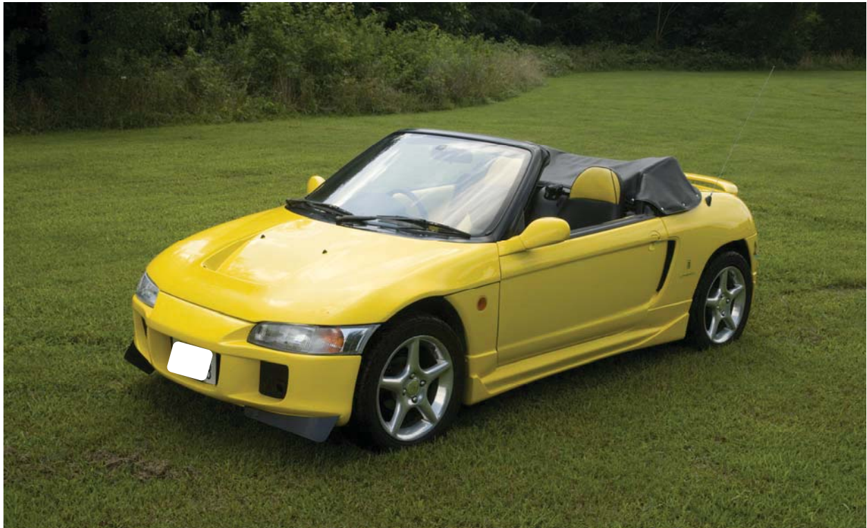
Frt bumper, hood & side skirts from 'Backyard'; Eagle 15" x 7" rims; Yoko 185R x 55 x 15 tires
