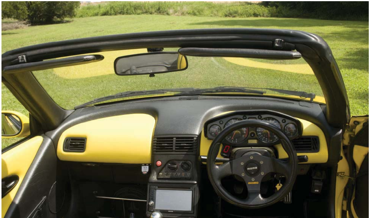
Hayabusa instrument cluster; gear indicator with ATRE; Kenwood receiver, amp & sound sys; heated seats; Clifford alarm
