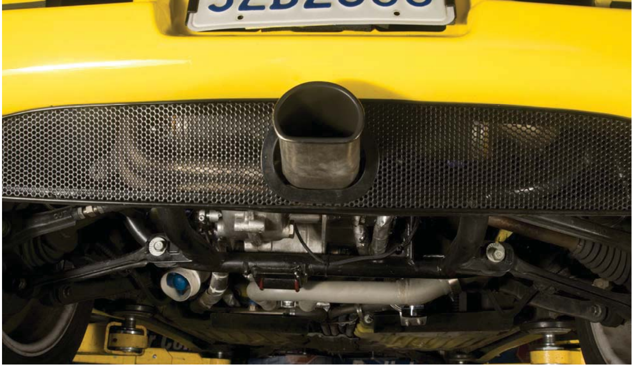
1300 Hayabusa with RageMotorsport drive assy and Quaife Diff w/ reverse & ltd slip; ceramic headers; ext oil sump & cooler; cres exhaust & Two Brothers muffler; JIT accessory drive assy runs alternator and AC pump; power commander ignition and quickshift; aux active and passive cooling sys
