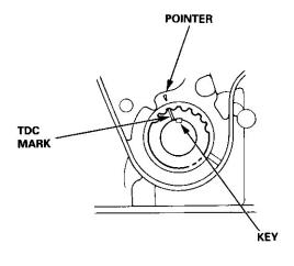
Set the camshaft pulleys so that the No. 1 piston is at TDC.
