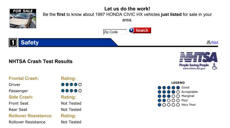
The National Highway Traffic Safety Administration (NHTSA) provides 3 different ratings - <u>full-width</u> <u>frontal crash test</u>, <u>side impact crash test</u>, and <u>rollover resistance</u>. The frontal crash test
