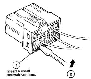
Lift up on the screwdriver and the lock will "snap" upward.
