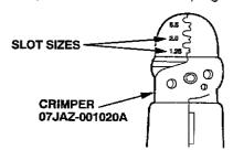
3. Strip the insulation off the end of the wire so the wire fits in the new terminal as shown. (If the wire has a wire seal, replace it with a new one from the kit.)
