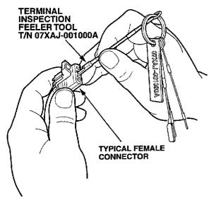
Compare the drag to the other terminals in the connector. If the drag is less, replace the terminal with a replacement terminal from the appropriate terminal repair kit.
