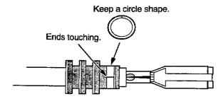
Inspect the quality of the wire crimp. If it has any of the following NO GOOD crimps, cut it off and start over.
