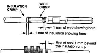
End of wire insulation 4. Position the terminal in the crimping tool slot with the solid portion of the terminal toward the anvil and the open section toward the former.
