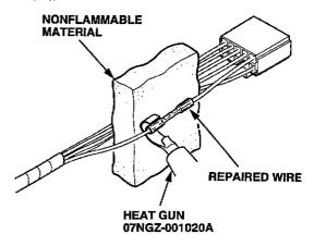
13. Plug in the heat gun, and turn it on. Start at the middle of the splice connector, and move the gun toward the ends as the tube shrinks. Apply heat evenly by rotating the curved heat spreader around the splice connector. Shrinking is complete when a small amount of sealant appears at each end of the tube.
