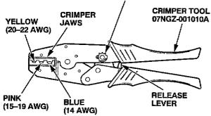
9. Insert one of the bare wires into the splice connector end that is in the crimper jaws. Push the wire all the way into the splice connector, and squeeze the crimper handles. Keep squeezing until the jaws touch, and hold it at that position until the ratchet clicks again.
