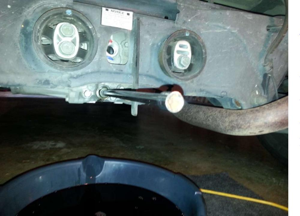
Step #5 – Once all of the Rear Differential Fluid has drained out into the Fluid Plan, take one of the new Crush Washers and place it on the clean <u>Drain Plug</u>. Then insert the Drain Plug (with the Crush Washer) into the Drain Plug hole tightening it fingertight (clockwise).
