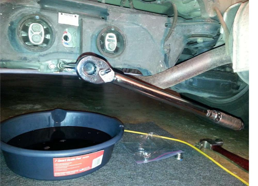
Step #6 – With the Torque Wrench attached to the extension which is inserted into the Drain Plug, set the torque wrench to 33 ft-lbs and tighten in a clockwise direction. Once 33 ft-lbs of tightening is achieved, remove the torque wrench and extension from the Drain Plug.
