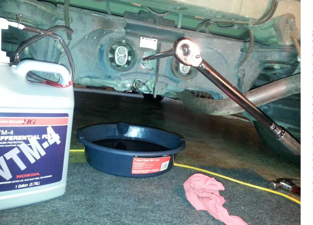
Step #8 – Once the differential is full, remove the tube and set the bottle aside. Then insert the Fill Plug with the new Crush Washer into the opening and tighten it finger-tight. Then insert the 1' extension into the square opening in the plug, connect your torque wrench to the extension, set the torque wrench to 33 ft-lbs, and tighten the plug in a clockwise direction. Once 33 ft-lbs of tightening is achieved, remove the torque wrench and extension from the Fill Plug.
