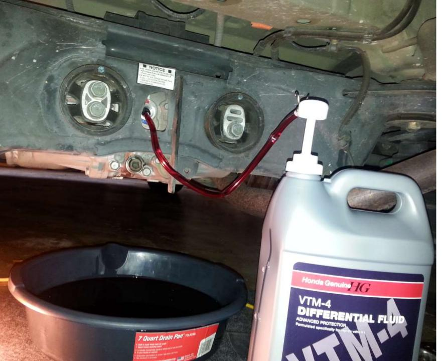
**Step #7** – At this point, get the VTM-4 Differential Fluid bottle and attach the Fluid Pump to it. Then, extending the upper tube of the pump into the Fill Plug opening, hand-pump about 3 quarts of differential fluid into the Rear Differential assembly.
