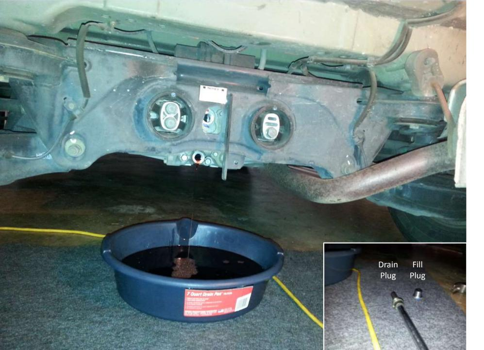
**Step #4** – With the upper Fill Plug removed and set aside, remove the lower <u>Drain Plug</u> and allow the Rear Differential Fluid to drain into the Fluid Drain Bowl.
