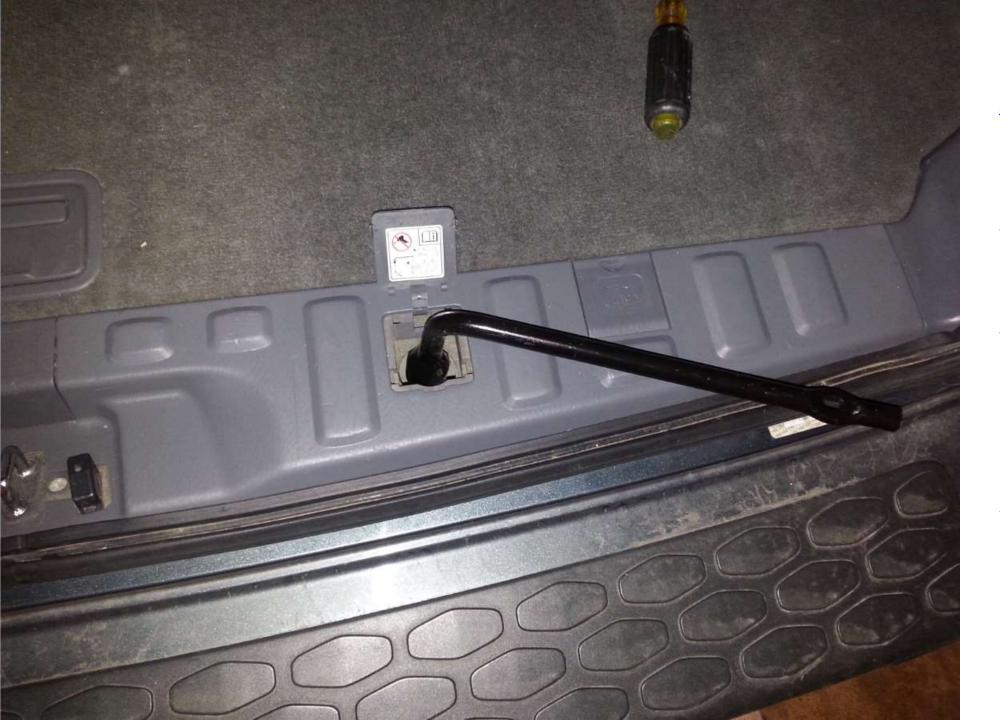
**Step #2** – Raise the rear hatch door and open the small plastic cover to the spare tire lowering mechanism. Insert the vehicle's lug wrench into the lowering mechanism (as shown) and rotate it counterclockwise to lower the spare tire.
