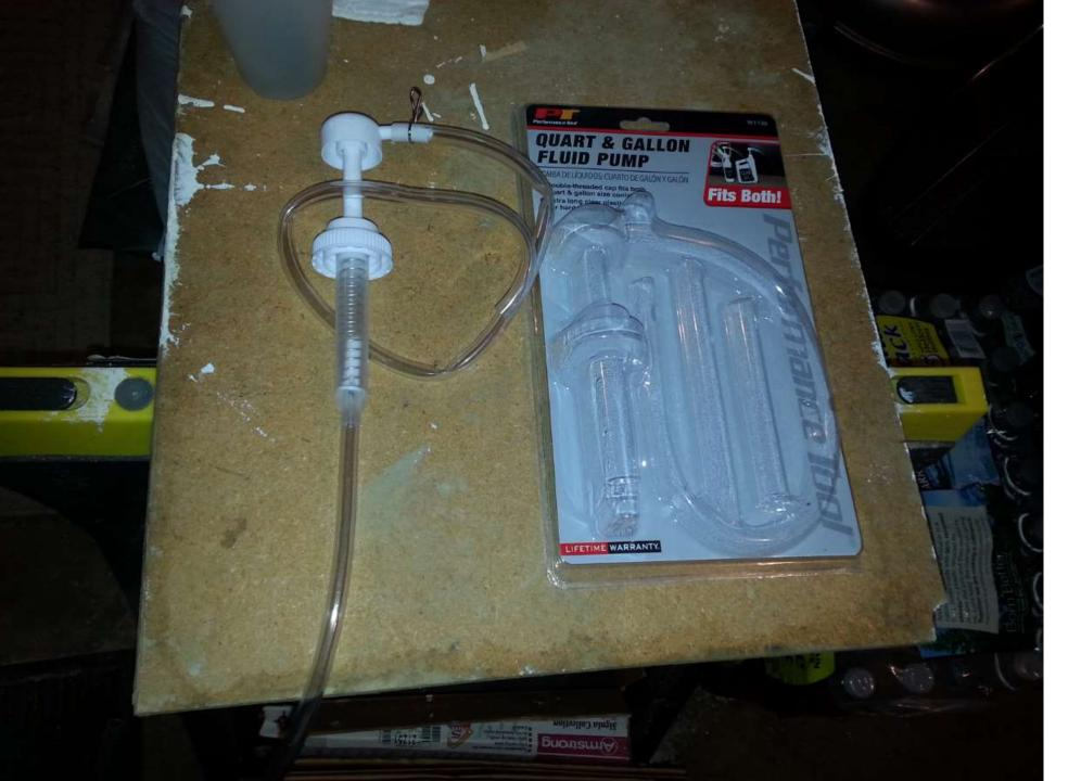
Supplies #2 – Another necessary item is the Fluid Pump and plastic hose that fits the 1-gallon Differential Fluid container.
