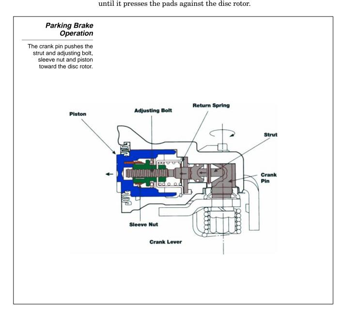
When the parking brake lever is released, the compressed Return Spring pushes the Adjusting Bolt and Piston back to their previous positions. As a result, the parking brake is released.
