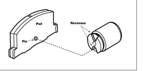
When brake pads are replaced, the piston with the sleeve nut must be forcibly rotated into the cylinder with the Special Service Tool shown below (SST 09719-00020).
