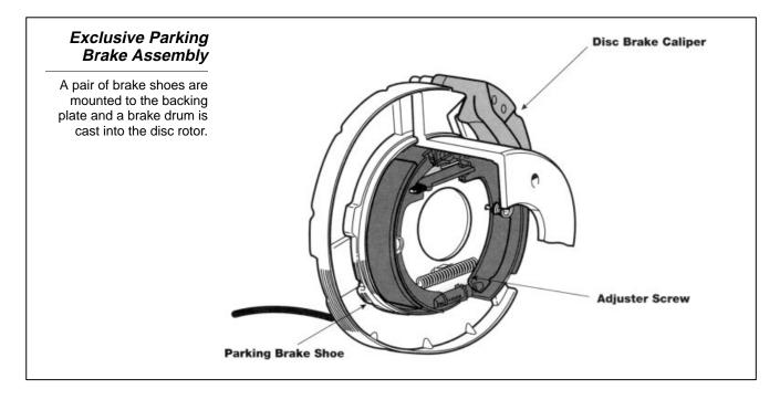
Activating the parking brake is similar to applying the parking brake on conventional drum brakes. Adjustment to the exclusive parking brake is done manually at the Shoe Adjusting Screw Set (Star Wheel) and must be done periodically.
