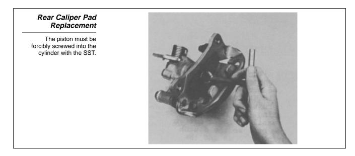
After pad replacement, the parking brake lever travel adjustment should be performed. Depress the brake pedal several times to activate the automatic adjustment within the caliper. Then adjust the cable for the proper number of clicks of the hand brake lever.
