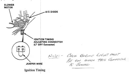
2. Connect the GRN and BRN terminals of the ignition timing adjusting connector (LT GRY) located at right, under dash with a jumper wire.
