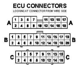
See ECU pin-out diagram above. Connector "A" is the largest. Connector "C" is the smallest.
