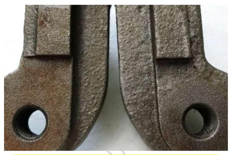
In the picture below, you can clearly see one bracket has been factory machined and the other has not been.
