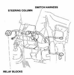
Attach the relay bracket to the steering column bracket using the 6 x 16 mm washer-bolt.
