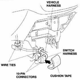
49. Plug the sub-harness 1-pin connector (routed in step 39) into the switch harness 1-pin connector (blue/red), then wrap one cushion tape around the connectors. Secure the connector to the vehicle harness using one wire tie.
