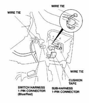
Secure the sub-harness and switch harness to the vehicle harness with two wire ties in the areas shown.
