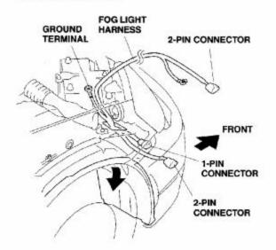
13. Behind the right headlight, remove and discard the bolt that fasten the fuse box bracket. Attach the fog light harness ground terminal and reinstall the fuse box bracket with a ground bolt from the kit.
