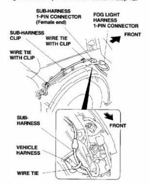
30. Secure the fog light harness to the vehicle harness with one wire tie in the area shown. Secure the sub-harness to the inner fender panel with two wire tie with clips from the kit, and with the one wire tie with clip attached to the subharness. Insert the clips into the empty holes in the inner fender panel.
