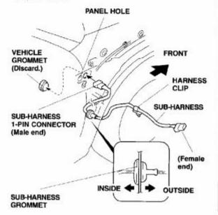
29. Route the female end of the sub-harness through the inner fender toward the front of the vehicle. Plug the sub-harness 1-pin connector into the fog light harness 1-pin connector routed in step 12.
