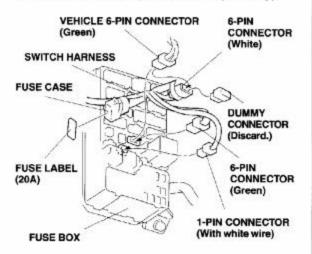
45. On A/T model, unplug the vehicle 6-pin connector (green) from the fuse box, and plug the green 6-pin connector from the switch harness into the fuse box. Plug the vehicle 6-pin connector (green) into the remaining 6-pin (green) connector on the fog light harness.
