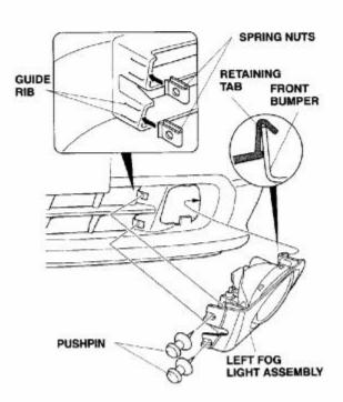
24. Fit the fog light assembly into position in the opening of the front bumper with the retaining tab behind the bumper. Using a pushpin, mark the bumper at each of the two mounting holes, then remove the fog light assembly.
