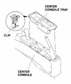
Remove the center console (two self-tapping screws, two washer-screws, and two clips). On M/T model, remove the shift knob.
