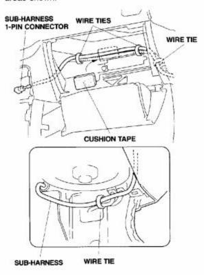
Get the switch harness. Route the switch harness under the dash, and over the steering column and the brake position switch harness.
