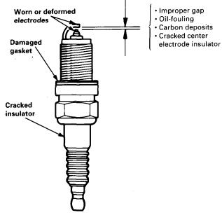
Burned or worn electrodes may be caused by:
