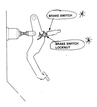
4. Screw in the brake switch until its plunger is fully depressed (threaded end touching the pad on the pedal arm). Then back off the switch 1/4 turn to make 0.3 mm (0.01 in) of clearance between the threaded end and pad. Tighten the locknut firmly Connect the brake switch connector.
