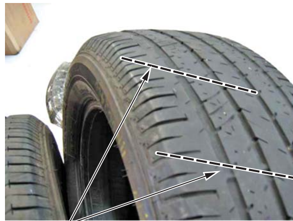
The tread is worn diagonally across the tire.
