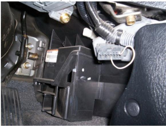
3. Jumper pins 4 and 9 of the Data Link Connector. See the photo above and the picture below. (Image courtesy of k-series.com)
