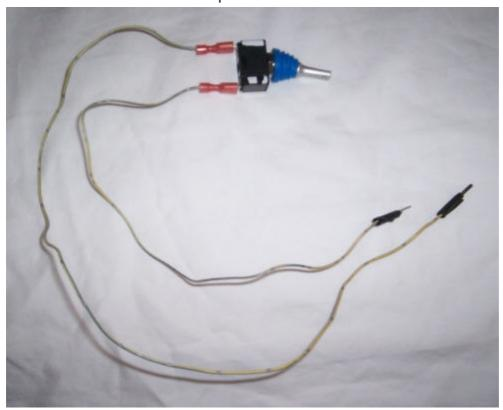
7. Insert the two male pins into the MES connector as needed to re-set the SRS system, per the instructions below.
