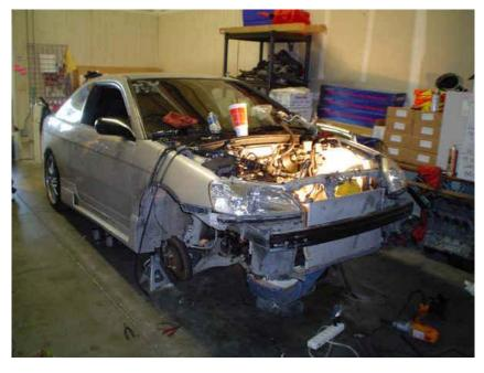
Now if you pulled the motor from the top. Jack the car back up so you have enough space to pull out the subframe. There are 4 bolts holding up your subframe. Take those 4 bolts out and the whole thing will drop.
