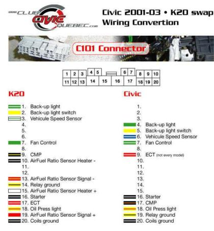
Note : The civic don't have AF Ratio sensor wired in the C101 connector. You must remake the complete wiring for this sensor. Just connect the wire of the RSX C101 directly to the sensor. On some car you should wire the Secondary O2 sensor and the O2 sensor heater relay for code free operation. The civic Sedan GX don't have the same wiring.
