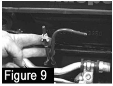
You have to gently bend the lines so that way it bends with the right line facing to the right and the left line is pointing towards the front of the engine bay. Now if you want to label these lines the left is the FUEL and the right one with the bend is the PURGE which hooks up to a vacuum on the manifold. Make sure you make no kinks in these lines or else you have to replace it somehow someway.
