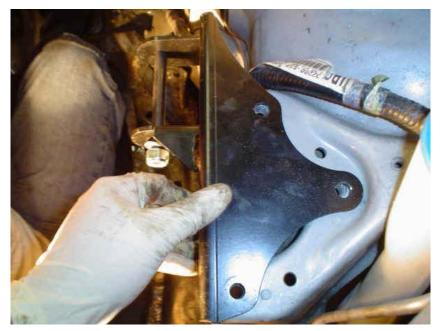
As you can see when the mount is flush to the frame the other 2 holes didnt line up perfectly. So basically what i did was i kept the bottom hole the same because that one lines up perfectly. The far right hole i had to grind it bigger up and to the left and the top one had to be grinded a little down and a little to the left.
