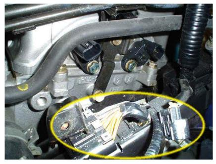
Lift up this plastic and it will reveal the radiator coolant temp sensor
