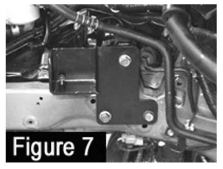
Now one thing you might notice is that the washers or spacers they give you will not make the bracket fit flush to the frame of the car. In fact you end up short on spacers. Pick up a bunch of spacers that look just like the ones they supplied so you can mount it flush.... Heres what i mean
