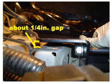
The bottom will mount flush except the top. I actually used the spacers on the bottom so it would be flush then didnt have any for the top. So check your package to see if they gave you more than 3 or 4 washers. If not then get a bunch more
