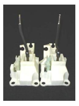
Here is a side by side comparison of the rsx-s (left) and the 01-05 civic (right)
