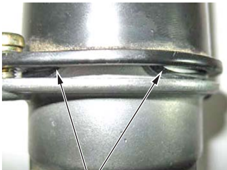
NO GOOD O-ring is pinched and/or rolled.
