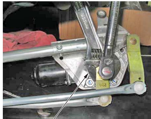
Hold the link while you tighten the nut. 31 N·m (23 lb-ft)
