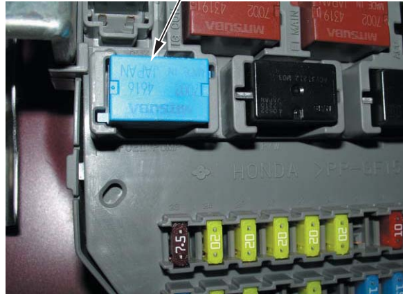
MITSUBA RELAY (Replace it if the vehicle is shown as eligible on a VIN status inquiry.)
