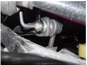
13. Position bar on end links and install nuts. Torque to 38Nm (28 lbf ft.) (Left side shown, repeat for right side)
