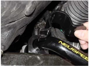
14. Install bracket over bushing and torque fasteners to 45 Nm (33 lbf ft.) (Right side shown, repeat for left side)
