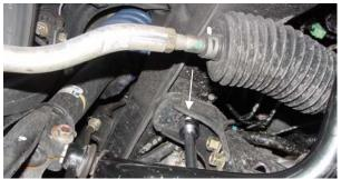
16. Install left center and right center sub-frame mounting bolts (19mm hex). Torque to 93 Nm (69 lbf ft.) (Left side shown, repeat for right side)
