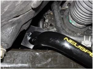
12. Using supplied grease, lube inner surface of bushing and install on bar. (Right side shown, repeat for left side)
