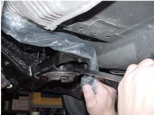
11. Leave protective cover on supplied anti-roll bar and install bar in reverse of removal. Remove protective cover once bar is in position.
