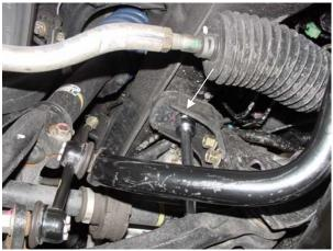
6. Remove left center and right center sub-frame mounting bolts (19mm hex).
