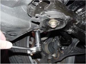
15. Raise sub-frame and install sub-frame bolt & bracket as shown. Torque bolt with 19mm hex to 93 Nm (69 lbf ft.) and bolt with 17mm hex to 103 Nm (76 lbf ft.) (Left side shown, repeat for right side)
