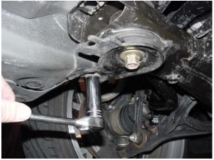
4. Remove left and right secondary sub-frame mounting bolts (19mm hex).
