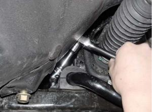
9. Remove bolts (14mm hex) securing anti-roll bar mounting bracket to sub-frame and remove brackets and bushings. NOTE: It may be helpful to use a 14mm hex socket and 3" extension to remove the rear mounting bolt as shown. (Right side shown, repeat for left side.)
