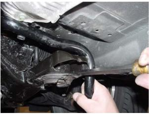
10. Remove bar from vehicle. NOTE: It may be necessary to pry sub-frame to one side to provide enough clearance to remove bar.
