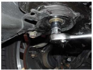
5. Remove left rear and right rear sub-frame mounting bolts (17mm hex).
