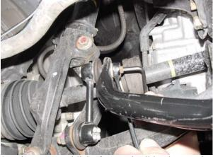
8. Disconnect end links from anti-roll bar by securing stud with 5mm hex key and loosening nut with 14mm wrench. (Left side shown, repeat for right side.)
