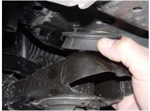
7. Slowly lower sub-frame and remove left rear and right rear rubber isolators.
