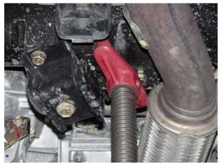
3. Support rear of sub-frame with a jack-screw or floor jack.
