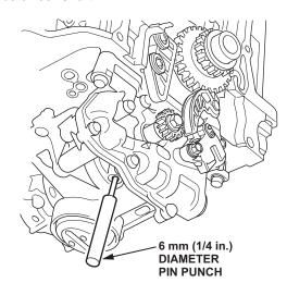
27. Loosen the oil pump sprocket mounting bolt.
