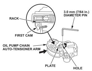
69. Apply new engine oil to the threads of the oil pump mounting bolts and the oil pump sprocket mounting bolt, then loosely install the oil pump with a new O-ring.
