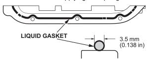
87. Install the cam chain case.
