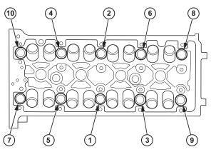
• After torquing, tighten all cylinder head bolts in two steps (90° per step) using the sequence shown above. If you are using a new cylinder head bolt, tighten the bolt an extra 90°.
