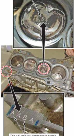
The "A" and "B" represents piston size. Piston sizes can be mixed in an engine block assembly.
