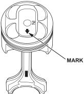
55. Set the piston in the ring compressor, and position the piston in the cylinder noting the rod/cap marks that you made in step 34.
