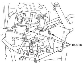
15. Disconnect the radiator hoses and the heater hoses. Disconnect the ATF warmer bypass hose (if equipped).
