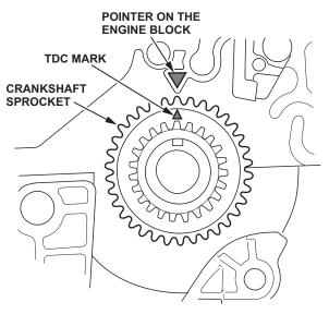
• Install the oil pump chain on the crankshaft sprocket with the colored link plate aligned with the TDC mark on the crankshaft sprocket.
