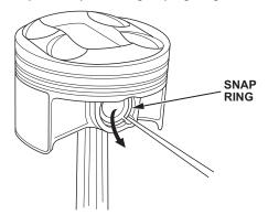
40. Put on gloves, heat the piston and the ends of the connecting rod to about 158°F (70°C), then remove the piston pin.
