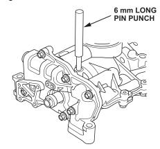
68. Turn the oil pump auto-tensioner plate counterclockwise to release the lock, then push the auto-tensioner arm, and set the first cam to the first edge of the rack. Insert a 3.0 mm (7/64 in.) diameter pin into the hole.
