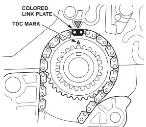
• Set the oil pump chain on the oil pump chain sprocket with the punch mark aligned with the center of the colored link plates, then install the oil pump chain sprocket to the oil pump.
