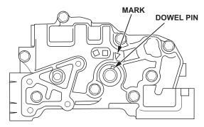
67. To hold the rear balancer shaft, insert the 6 mm (1/4 in.) diameter long pin punch into the maintenance hole in the balancer shaft holder and through the rear balancer shaft.
