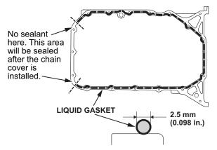
78. Install the oil pan to the engine block.
