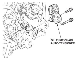
29. Remove the oil pump sprocket and the oil pump.
