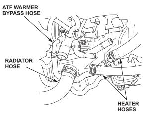
16. Remove the two bolts securing the connecting hose. Disconnect the water bypass hose.
