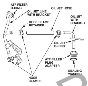
8. Install the oil jet line on the ATF hose with a new hose clamp.
