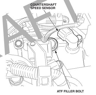
3. Remove the countershaft speed sensor. *For Odyssey*, refer to the 1999–04 Odyssey Service Manual, page 14-134. *For Pilot*, refer to the 2003–04 Pilot Service Manual, page 14-123.
