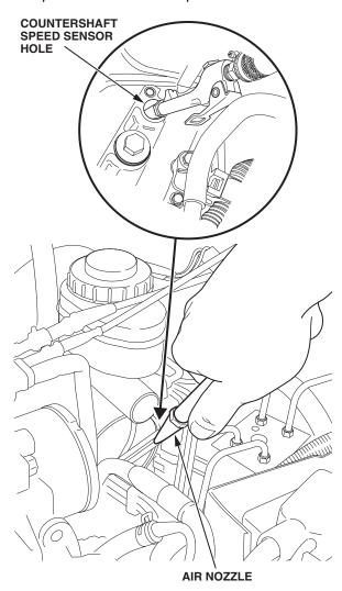
5. Using a clean shop towel, wipe out the bore of the countershaft speed sensor hole.
