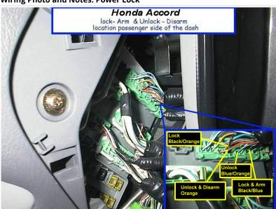
On LX models, can also use black/white (-) in a gray 2 or 3 pin plug by the front of the driver side fuse box.
