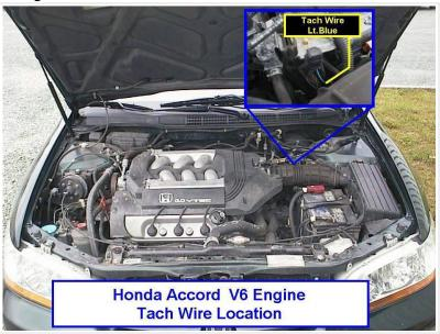
The tach test connector is located behind the battery on the 4 cylinder, and on a bracket attached to the drivers side strut tower on the 6 cylinder motor. The tach test connector is a white 2 pin connector, and may be covered by a black rubber boot.
