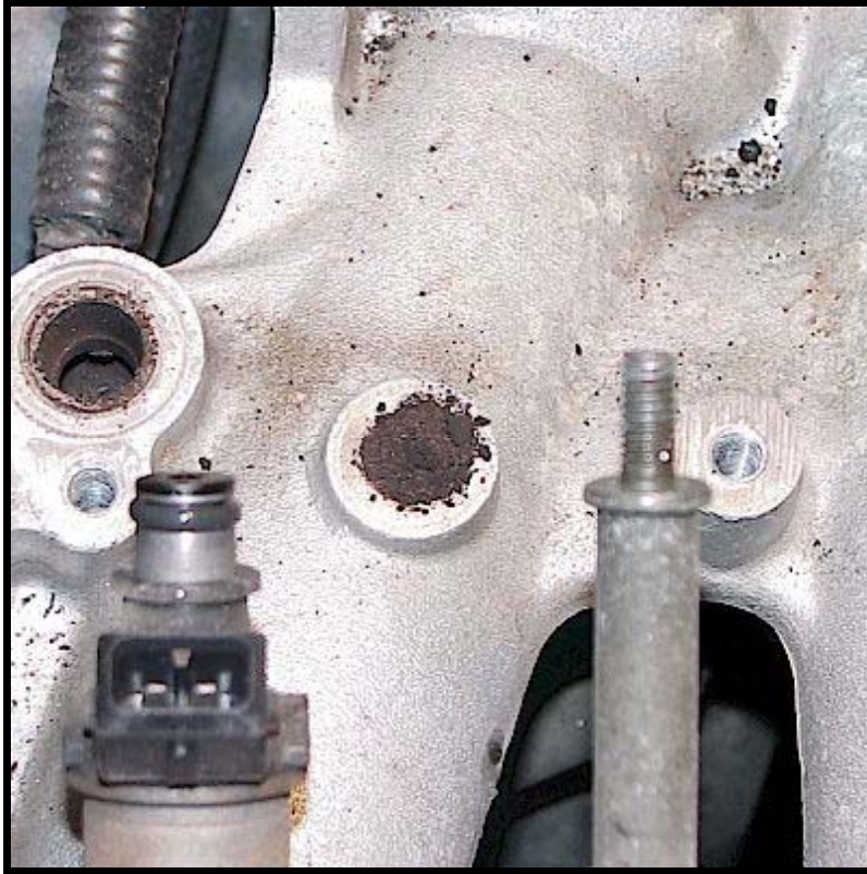
Image 1-13 Close Up of Clogged EGR Port
