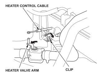
14. *Under the dashboard:* Reconnect the air mix control cable end to the arm. Push the heater control arm to its maximum cold position.
