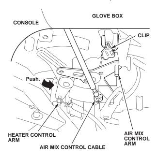
19. Pull on the air mix control arm to make sure the air mix doors are closed; then pull back on the air mix control outer cable to remove the slack in the inner cable, and snap the outer cable into the retaining clip.
