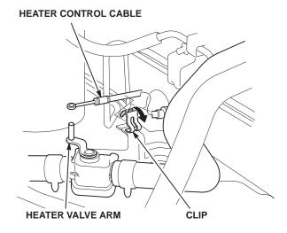
18. *Under the dashboard:* Reconnect the air mix control cable end to the arm. Push the heater control arm to its maximum cold position.
