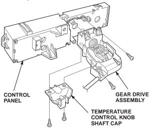
10. Turn the temperature control knob to maximum cold. The drive and driven gears will disengage. Align the long tooth on the drive gear to the short tooth on the driven gear.
