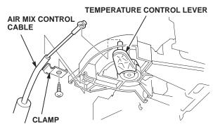
13. Install a new air mix control cable (see PARTS INFORMATION) on the temperature control lever. Make sure the outer cable is behind the stop, then tighten the clamp screw. Rotate the temperature control knob to maximum cold.
