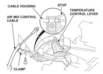
9. Remove the air mix control arm. Apply DC111 grease to the areas shown. Also apply grease to the slots on the other arms that mate to the shafts on the air mix control arm.
