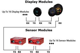
Remove termination jumpers from all sensor modules excluding sensor module furthest from display modules.
