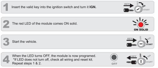
\*To RESET, press and hold button and plug in module. LED comes on. When LED goes off, release button.
