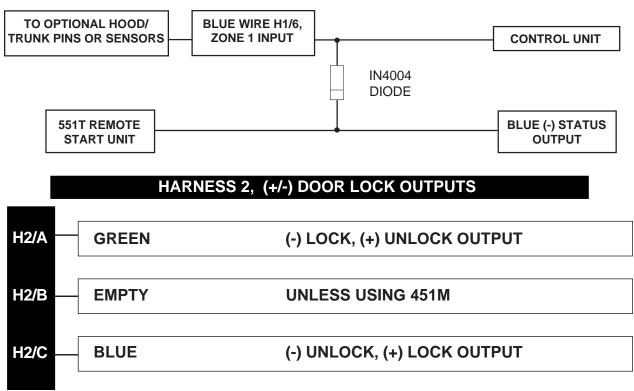
This system can control two common power door lock types without any additional parts! With certain vehicles, or if an actuator is to be installed, either a 451M Door Lock Relay Satellite or two relays will be required.
