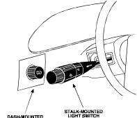
5. If it does return to zero, turn the parking lights back on and, using the dash light dimmer control, turn the brightness of the dash lights up and down. If the meter changes more than a volt when using the dimmer, look for another wire. If it stays relatively close to (+)12V, you have found your parking light wire.
