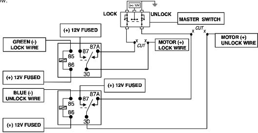
**Important!** If these are not connected properly, you will send (+) 12 volts directly to (-) ground, possibly damaging the alarm or the factory switch.
