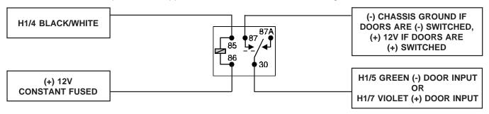
**H1/5 GREEN** (-) door trigger or **H1/7 VIOLET** (+) door trigger input: If the door switch wire you found is (-) when the door is open, connect the GREEN wire to it. If the door switch wire you found is (+) when the door is open, use the VIOLET wire instead.
