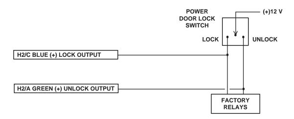
**IMPORTANT!** Remember that functions of these wires reverse between Type A and Type B!
