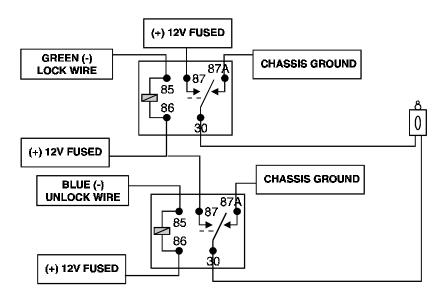
**IMPORTANT!** Do not connect the outputs of the alarm directly to the actuator!
