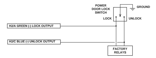
IMPORTANT! Remember that functions of these wires reverse between Type A and Type B!
