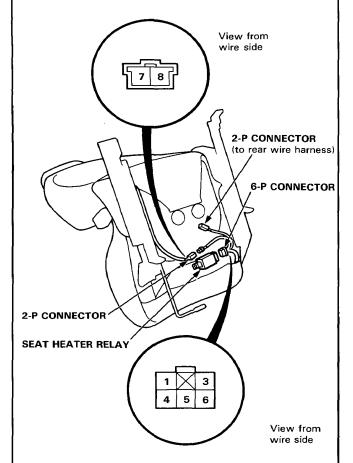
Check for continuity between the No. 1 and No. 5 terminals, and between the No. 7 and No. 8 terminals (R x 10<sup>3</sup> scale)
